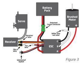
ESC) is not used. After calibration (See "How to Calibrate the ESC", page 10), you may need to swap the two motor wires to get the wheels to spin in the right direction.
